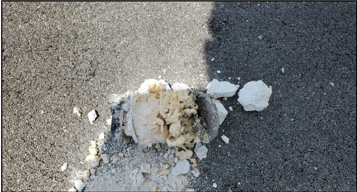
Photo 13: Sample 6 collected from area 2. Underlying roof could not be cored as the asphalt bound the coring tool
